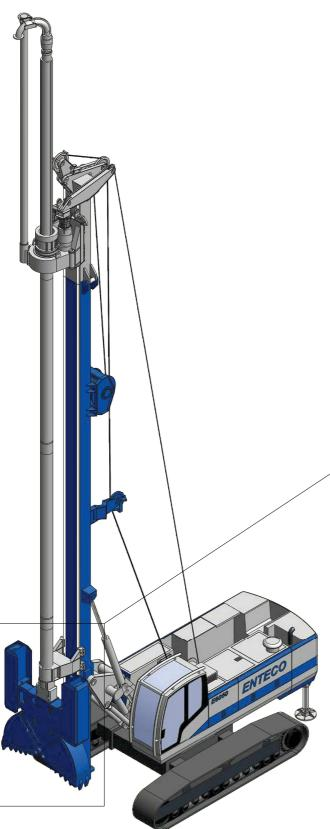
The diaphragm wall grab is mounted on the Kelly of the SP Kit instead of the standard tool
