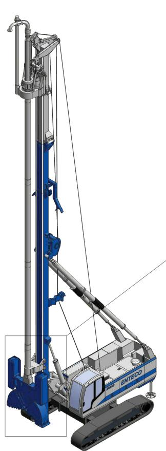
The diaphragm wall grab is mounted on the Kelly of the SP Kit instead of the standard tool
